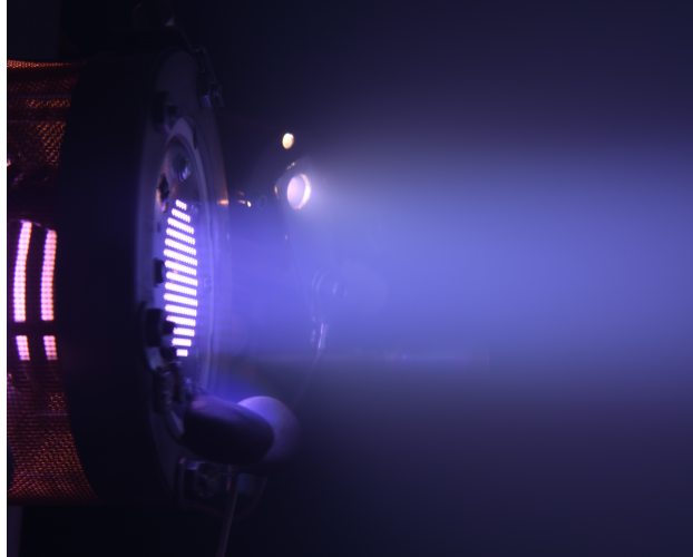
Fig. 7 Photo of the thruster operating on argon propellant with a shielded filament neutralizer. The version shown included capacitors on the grids to reduce RF pickup, but were removed in later versions.
