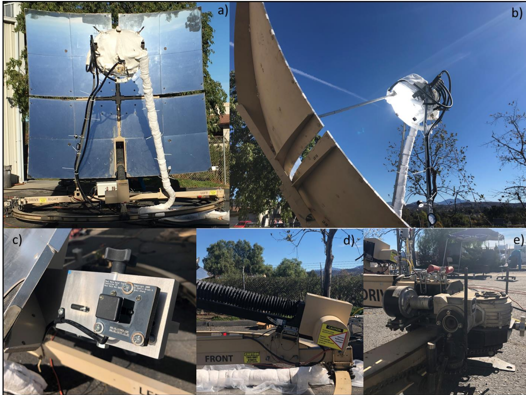
Figure B-6. Key components of the on-sun CSP system: (a) parabolic mirrors, (b) concentration of solar energy at the receiver, (c) photosensor, (d) vertical drive, and (e) horizontal drive.
